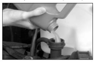
Fill the radiator with the proper DEX-COOL<sup>®</sup>
